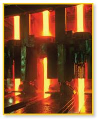
The rotary caster is one of Gerdau's most sophisticated processes. It begins with molten steel from the ladle teemed through a ceramic shroud into the tundish. From the tundish, steel enters the rotating mold through a pouring nozzle and is shrouded with an inert gas to maintain the steel's microcleanliness by avoiding reoxidation.
