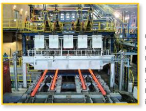
Our strand caster uses advanced technologies to produce clean steel with a homogenous internal structure.
