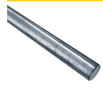
Gerdau's quench and tempered bars are produced through an advanced induction heat treating and proprietary quench process that treats each bar individually. The process adds strength and improves resistance to impact and abrasion. Gerdau's quench and tempered bars enable customers to machine distortion-free parts, eliminate production processes, such as stress relieving or straightening, and save money. Quench and tempering can be done to all heat treatable grades of carbon and alloy steels.
