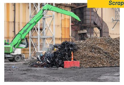
Our steelmaking process begins with the highest quality blend of recycled scrap steel. The use of steel scrap as a raw material reduces energy consumption in our production process, and also minimizes emissions of CO2.
