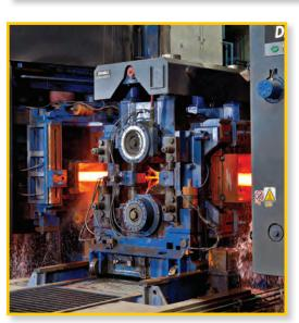
Included in this capital expenditure project is the installation of six additional rolling mill stands. These new stands allow us to increase the input bloom sizes up to 280mm squares and offers higher reduction ratios. Enhancements to the cooling beds and the installation of two hot abrasive saws are also part of this project.
