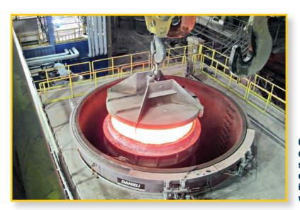
Our state-of-the-art continuous caster was commissioned in October 2012. The new strand caster transforms liquid steel into solidified steel billets for subsequent re-rolling. This caster features a 10 meter radius, four cooling zones and complete shrouding from ladle to mold with automated mold level control and electromagnetic stirring. The caster has the capability to produce billets and blooms in 152mm, 210mm and 280mm square dimensions.
