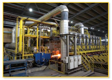
Our new walking beam reheat furnace features six zones with top and bottom firing at the pre-heat, heat and soak stations. The new furnace increases reheating capacity and offers capability to reheat billets and blooms from 152mm to 280mm square sections. The automatic controls allow for custom reheating temperature curves for individual order requirements and adjustable residence time for improved decarburization.
